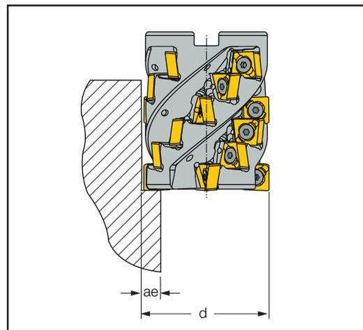
Fig. 11 Slab milling and milling deep shoulder
