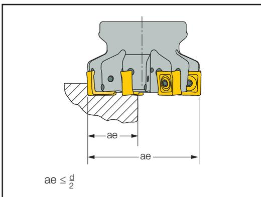
Fig. 12 Face milling with depth of cut no more than the radius of a milling cutter
