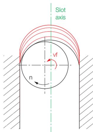
Solid carbide endmills (SCEM), which are used in machining titanium, can be successfully operated by trochoidal milling techniques and commonly feature 4-5 flutes. A variety of SCEM with greater number of flutes have been designed specifically for trochoidal milling applications. Table 29 gives basic data about ISCAR's families of these solid carbide endmills.
