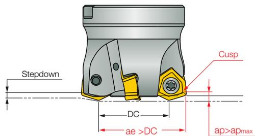
**Fig. 20** Width of cut and cusps in fast feed milling
