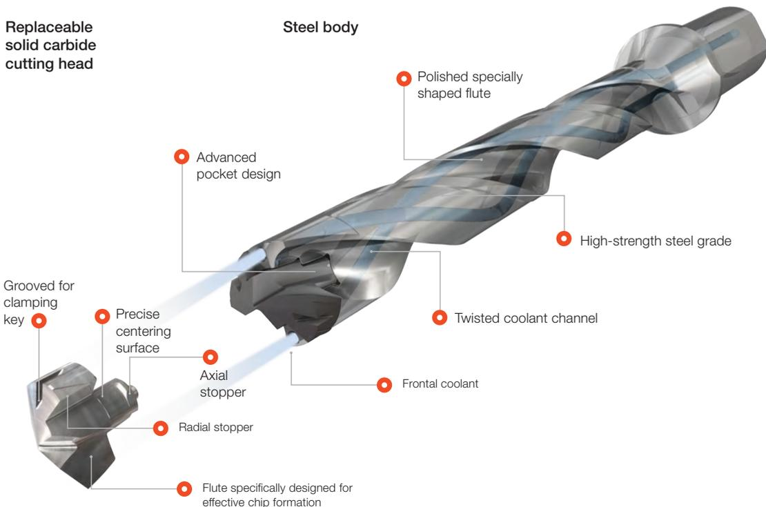
Fig. 29 The structure of a SUMOCHAM drill
