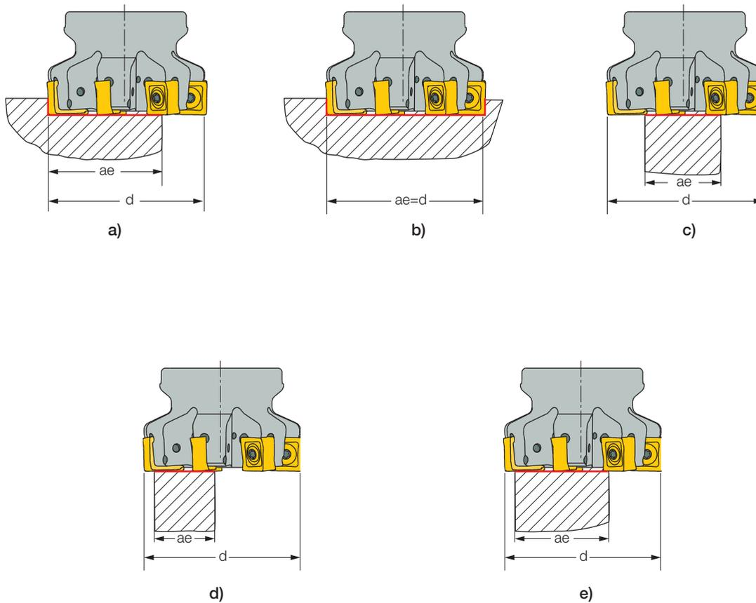
**Fig. 13 Possible application of 90° face mills**
