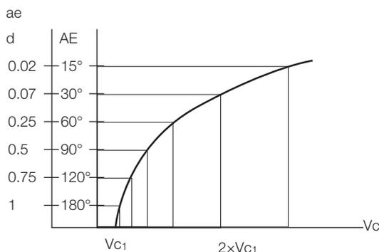
Fig. 8 Plot Vc against AE and ae
