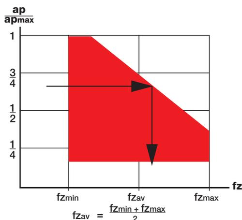
Fig. 14 A typical field of feeds in face milling for  $a_e=(0.6...0.8) \times d$
