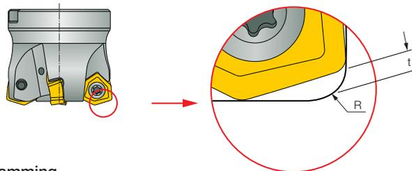
**Fig. 21** Radius for programming
