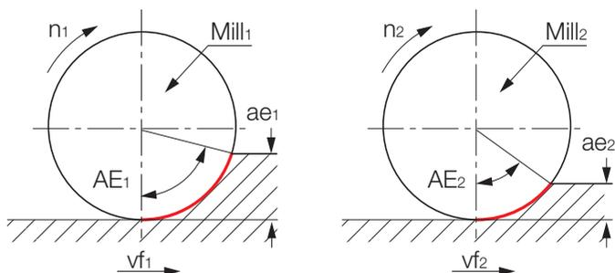
**Fig. 7** Contact arc and angle of engagement
