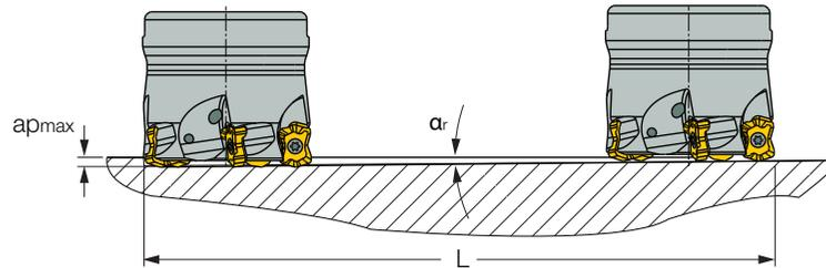
Fig. 22 Ramp-down milling
